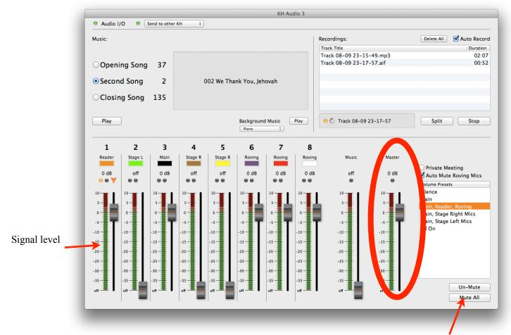
The master **Mute All** button can be held down with the mouse to temporarily mute all signals flowing through the system. As soon as you let the mouse button go, the master will return to its previous level. This is very useful when attendants are adjusting the microphones on stage. Hold it while they are moving the mikes to avoid unwanted sounds through the system. You can also do this by holding down the **[M]** key on the keyboard.
